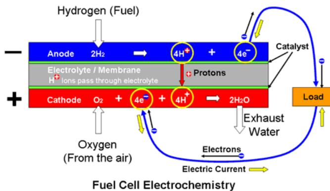
Figure 2: Chemical reaction within a fuel cell (Woodbank Communications Ltd, u.d.)
