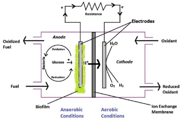
Figure 4: Microbial Fuel Cell (MFC) (Deeksha, p.121, 2013)
