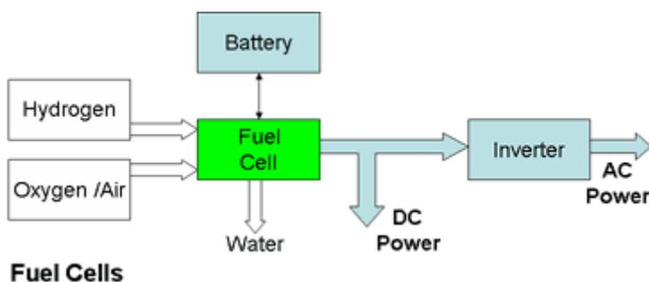
Figure 1: Principle of the fuel cell (Woodbank Communications Ltd, u.d.)
