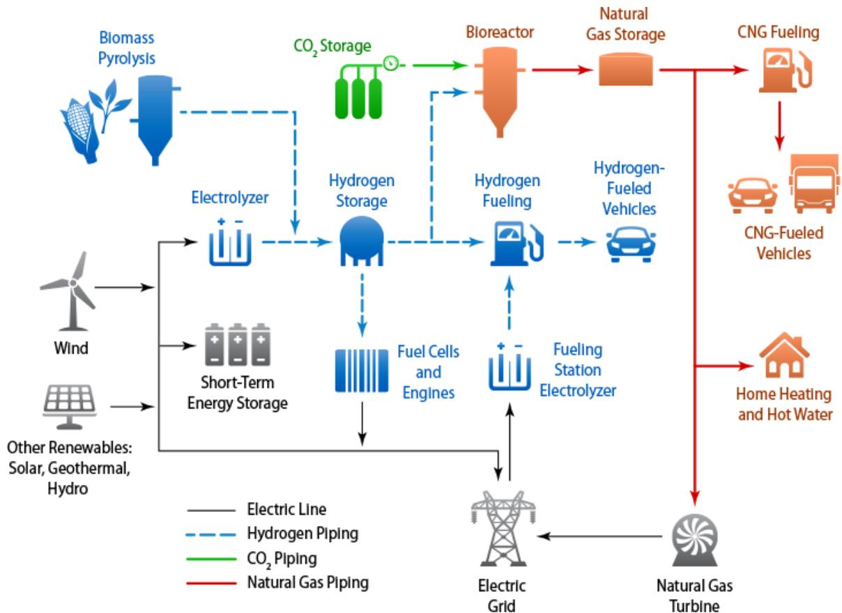
Figure 6: diagram with different solution to use hydrogen (NREL, 2011)
